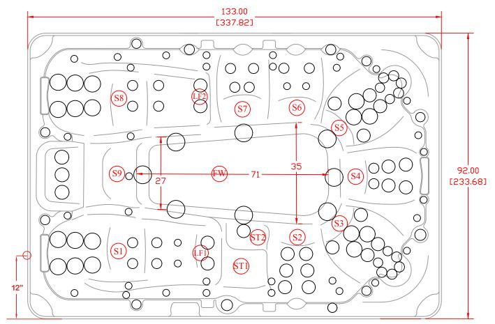
Place Electrical Supply on left side of Hot Tub. (12" to the rear of spa)
