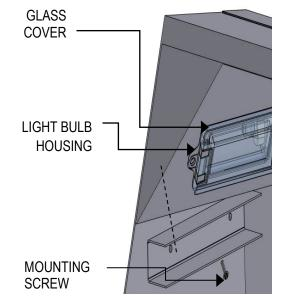
**4)** Using a soft cloth or paper towel, replace new light bulb into the housing (fingerprints left on the bulb may reduce its life). Make sure the metal prongs on the light bulb slip into the openings in the light housing
