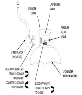
16) TO CONNECT TO LP TANK, ATTACH THE BLACK COUPLING NUT ON THE REGULATOR ASSEMBLY TO THE LP TANK BY ROTATING CLOCKWISE DIRECTION (SEE ILLUSTRATION BELOW) UNTIL IT IS COMPLETELY THREADED ONTO THE CYLINDER VALVE BEFORE TURNING GAS SUPPLY ON. TO REMOVE TURN THE BLACK COUPLING NUT OF THE HOSE AND REGULATOR ASSEMBLY IN A COUNTER- CLOCKWISE DIRECTION.
