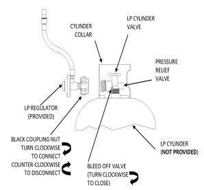
16) TO CONNECT TO LP TANK, ATTACH THE BLACK COUPLING NUT ON THE REGULATOR ASSEMBLY TO THE LP TANK BY ROTATING CLOCKWISE DIRECTION (SEE ILLUSTRATION BELOW) UNTIL IT IS COMPLETELY THREADED ONTO THE CYLINDER VALVE BEFORE TURNING GAS SUPPLY ON. TO REMOVE TURN THE BLACK COUPLING NUT OF THE HOSE AND REGULATOR ASSEMBLY IN A COUNTER- CLOCKWISE DIRECTION.
