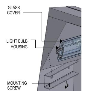
4) Using a soft cloth or paper towel, replace new light bulb into the housing (fingerprints left on the bulb may reduce its life). Make sure the metal prongs on the light bulb slip into the openings in the light housing
