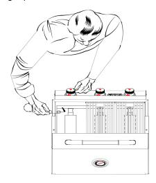
Burner should light immediately. If more than one burner is needed, repeat procedure with each burner.
