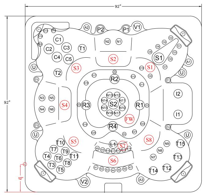
Place Electrical Supply on left side of Hot Tub. (12" to the rear of spa)
